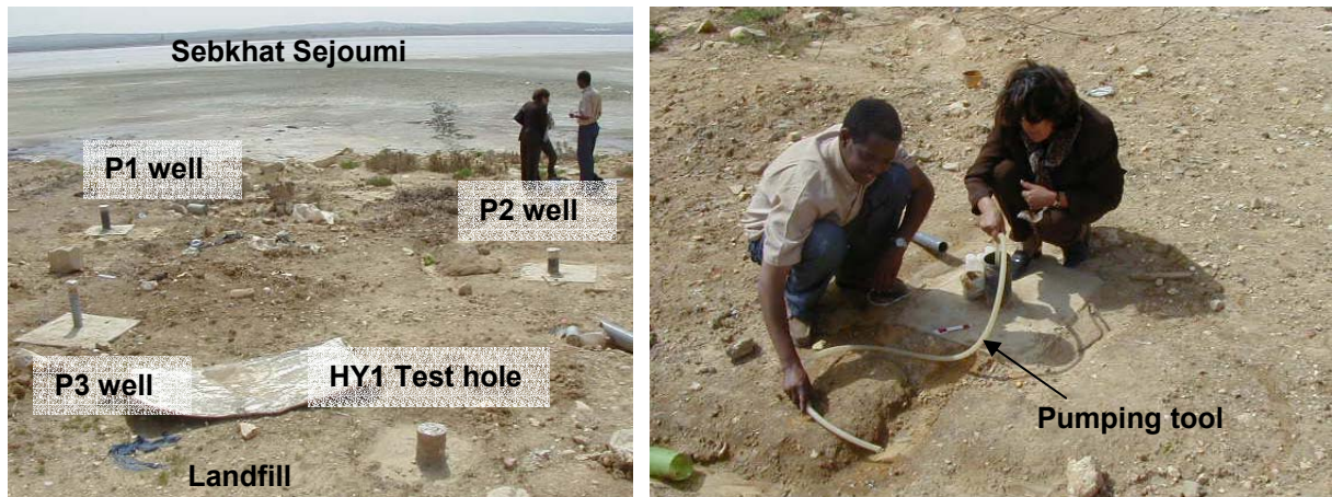
Plate 1: Field photograph of the observation wells HY1-P1, P2, P3, and HY1 test hole (left) and an operation of groundwater sampling by hand pumping tool (right).
